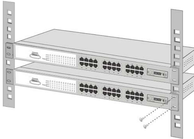
Figure 2-6. Mount the switch in an EIA standard 19-inch Rack
